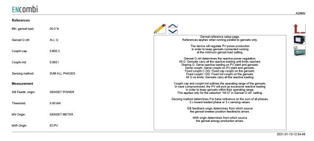
ECpv will regulate PV power production in order to keep gensets connected running at the minimum genset load setting.
