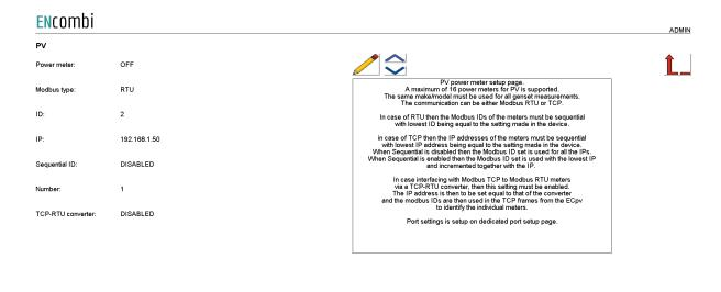
A maximum of 16 power meters for PV is supported. The same make/model must be used for all PV measurements. The communication can be either Modbus RTU or TCP. Check the link below to see which meters are supported by ECpv. <a href="http://www.encombi.com/products/ecpv/">http://www.encombi.com/products/ecpv/</a>
