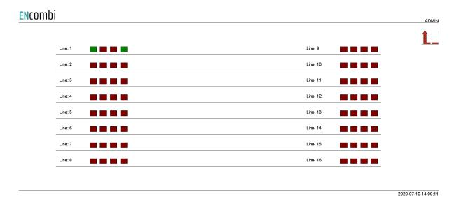
Each builder line consists of four gates. The status of the gates are represented by the color. Red means that the gate is false and green that the gate is true.
