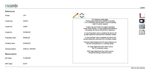
The inverter protocol itself to select in the ECpv slaves is determined by the make/model of inverters inside their respective inverter clusters.
