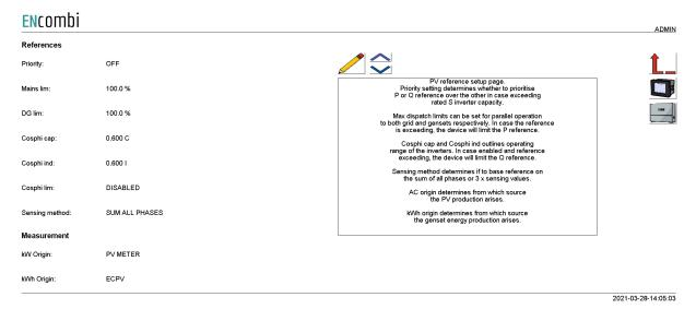
Priority setting determines whether to prioritize P or Q reference over the other in case exceeding rated S inverter capacity.
