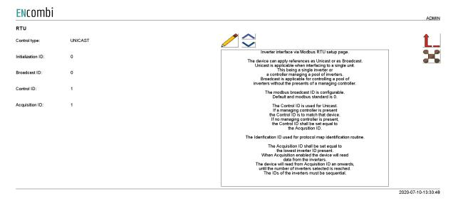
The ECpv can apply references as Unicast or as Broadcast. Unicast is applicable when interfacing to a single unit. This being a single inverter or a controller managing a pool of inverters. Broadcast is applicable for controlling a pool of inverters without the presence of a managing controller.
