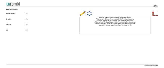
Here the sensitivity of the Modbus Master communication alarms can be adjusted. The settings dictates the number of timeouts to encounter before the respective Modus Master alarm is raised.
