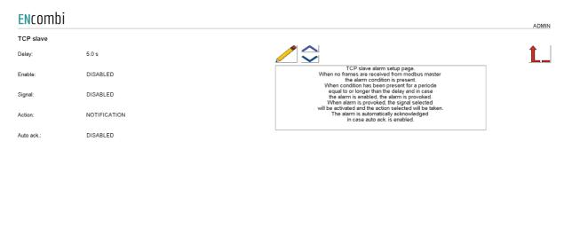
When no frames are received from modbus master the alarm condition is present. When the condition has been present for a period equal to or longer than the delay and in case the alarm is enabled, the alarm is provoked. When the alarm is provoked, the signal selected will be activated and the action selected will be taken. The alarm is automatically acknowledged in case auto ack. is enabled.
