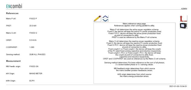
Mains P ctrl determines the active power regulation scheme.
