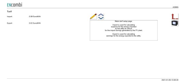
Import is used for calculating expense for the energy imported by the utility as well as for the import savings generated by the PV plant.
