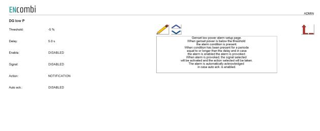
When the genset power is below the threshold the alarm condition is present. When the condition has been present for a period equal to or longer than the delay and in case the alarm is enabled the alarm is provoked. When the alarm is provoked, the signal selected will be activated and the action selected will be taken. The alarm is automatically acknowledged in case auto ack. is enabled.
