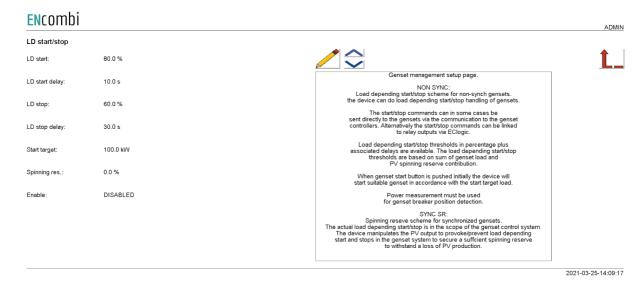
The ECpvh can do load depending start- and stop handling of gensets for two types of genset systems.
