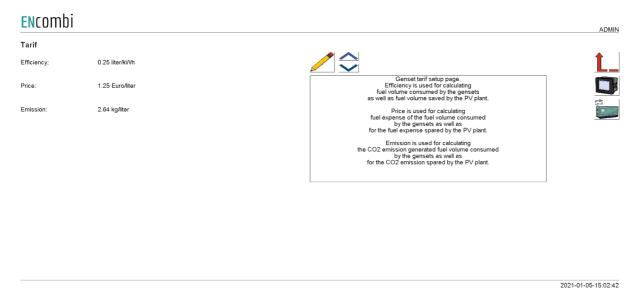
Efficiency is used for calculating fuel volume consumed by the gensets as well as fuel volume saved by the PV plant.
