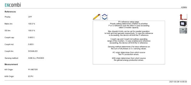
Priority setting determines whether to prioritise P or Q reference over the other in case exceeding rated S inverter capacity.
