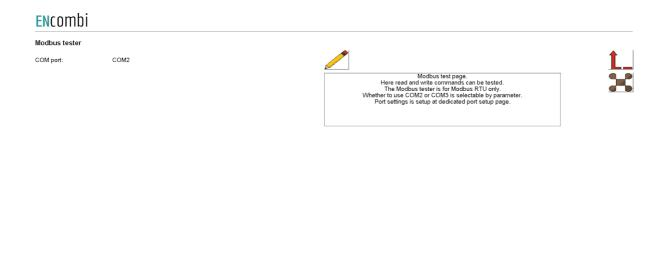
Afterwards clicking on the Modbus Tester button on the right hand side leads to the Modbus Tester itself where Modbus RTU read and write commands of various length and function codes can be transmitted and the response received is shown.
