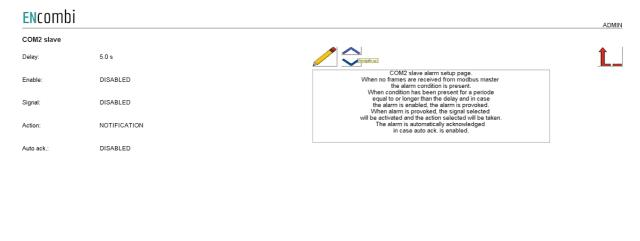
When no frames are received from modbus master the alarm condition is present. When the condition has been present for a period equal to or longer than the delay and in case the alarm is enabled, the alarm is provoked. When the alarm is provoked, the signal selected will be activated and the action selected will be taken. The alarm is automatically acknowledged in case auto ack. is enabled.
