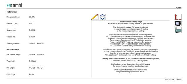
ECpvh will regulate PV power production in order to keep gensets connected running at the minimum genset load setting.
