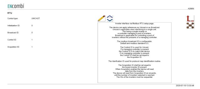
The ECpvh can apply references as Unicast or as Broadcast. Unicast is applicable when interfacing to a single unit. This being a single inverter or a controller managing a pool of inverters. Broadcast is applicable for controlling a pool of inverters without the presents of a managing controller.
