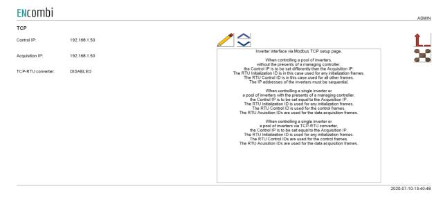
When controlling a pool of inverters, without the presence of a managing controller, the Control IP is to be set differently than the Acquisition IP.
