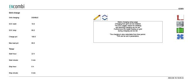
When parallel with the grid it is possible to charge the battery from the grid. The following options are available:
