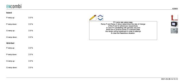
Ramp P and Ramp Q down determine the rate of change of the P and Q references respectively. Unique ramp rates are available for Island and Grid-tied operation respectively. In case PV parallelling with gensets only and these are in reverse power or overload state the ramps will be bypassed in order to attempt to clear the hazardous situation.
