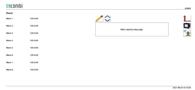
A total of 16 utility connections are supported. Above page is one of two pages available for setting up the rated mains trafo sizes.
