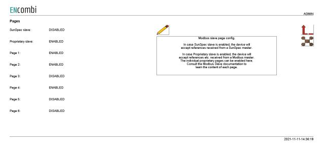
In case SunSpec slave is enabled, the ECpvX will accept references received from a SunSpec master. In case disabled the reference will be generated by the ECpvX's own setup found under genset or mains settings depending on whether parallelling to genset or mains is ongoing.
