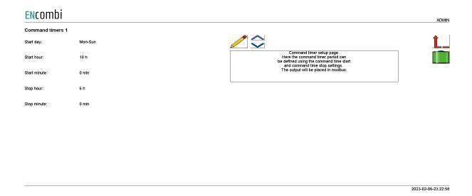
It is possible to set up 4 command timers. Type in the start day and time and stop time for the command timer. The output will be available on modbus and can be used for EClogic status/commands.
