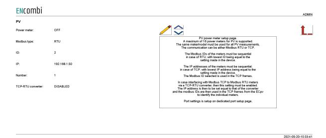
A maximum of 16 power meters for PV is supported. The same make/model must be used for all PV measurements. The communication can be either Modbus RTU or TCP. Check the below link to see which meters are supported by ECpvX. http://www.encombi.com/products/ECpvx/
