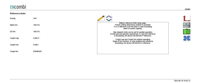
Priority setting determines whether to prioritize P or Q reference over the other in case exceeding rated S inverter capacity.
