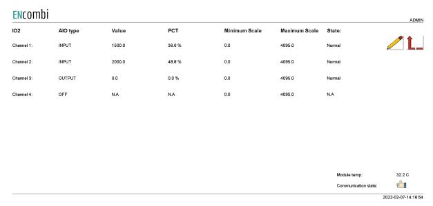
From this page it is possible to scale the input/output on each channel of the IO module. The input value can be used for Pref, Qref or other data points. This is set in EClogic. The value shown is the scaled value and the percentage is the percentage of the range from 0-100%. The maximum range is 0-4095.
