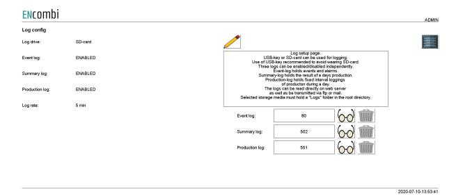
A new Event log is generated every day. The event log holds entries of any events taking place or any occurrences of alarms on that particular day. All entries are time stamped. The ECpvX can be set up to notify by email when a new entry is made in the event log. The ECpvX will in the text include the six most recent entries in the log.
