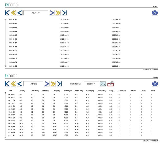
Note that the column heading of the production log shown is not actually included in the actual file being sent by email or transferred by FTP. The files only contain the data itself.
