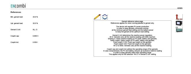
The ECpvX will regulate the PV power production in order to keep gensets connected running at the minimum genset load setting. The ECpvX will regulate the battery power production in order to keep gensets connected running at the optimum genset load setting.
