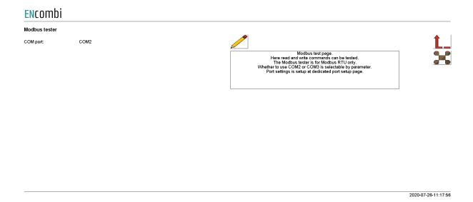
Afterwards, clicking on the Modbus Tester button on the right hand side leads to the Modbus Tester itself where Modbus RTU read and write commands of various length and function codes can be transmitted and the response received is shown.
