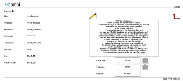
When using an installer/customer hosted database the data visualization part is in the scope of the installer/customer as well. The data to push is configurable according to the MySQL documentation on ENcombi website:
