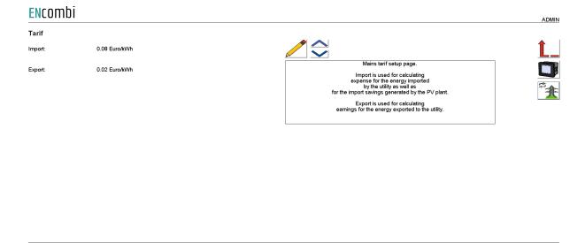
Import is used for calculating expense for the energy imported by the utility as well as for the import savings generated by the PV plant.
