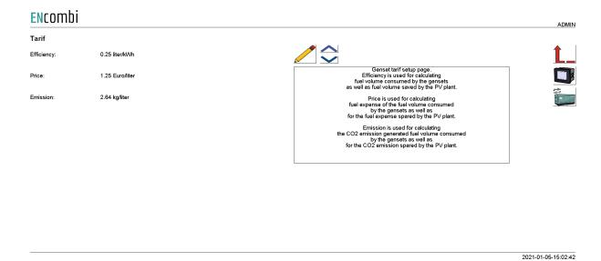
Efficiency is used for calculating fuel volume consumed by the gensets as well as fuel volume saved by the PV plant.
