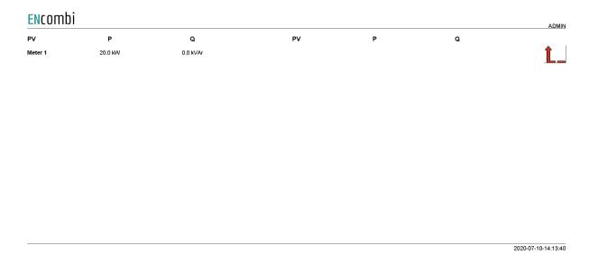
Clicking on a PV meter label, "Meter1" being the only option in the above example, will lead to a page with more detailed information about that specific PV meter.
