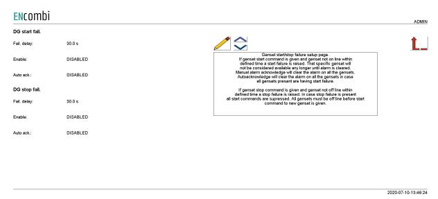
If the genset start command is given and a genset is not on line within defined time a start failure is raised. That specific genset will not be considered available any longer until the alarm is cleared. Manual alarm acknowledgment will clear the alarm on all the gensets.
