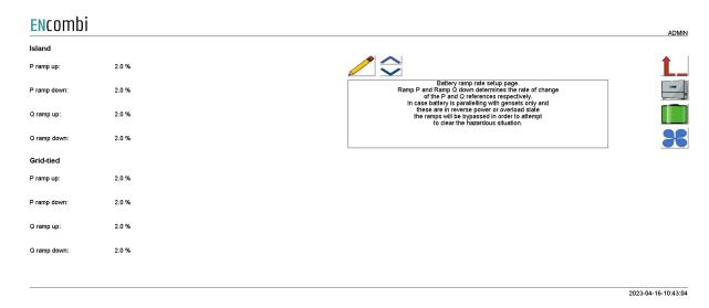
Ramp P and Ramp Q down determine the rate of change of the P and Q references respectively. Unique ramp rates are available for Island and Grid-tied operation respectively. In case battery parallelling with gensets only and these are in reverse power or overload state the ramps will be bypassed in order to attempt to clear the hazardous situation.
