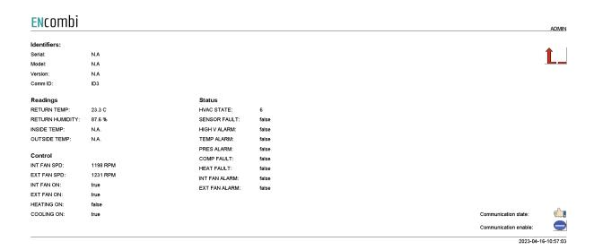
In the lower right corner communication status for the HVAC is shown. In case the HVAC is failing to communicate for whatever reason, communication to that specific inverter can be disabled and enabled again at a later stage on the start/stop button.
