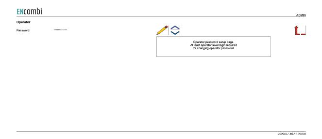
On the same submenu level the set up pages for tailoring access level required for executing various commands are found. Clicking the up/down arrows will lead to them.
