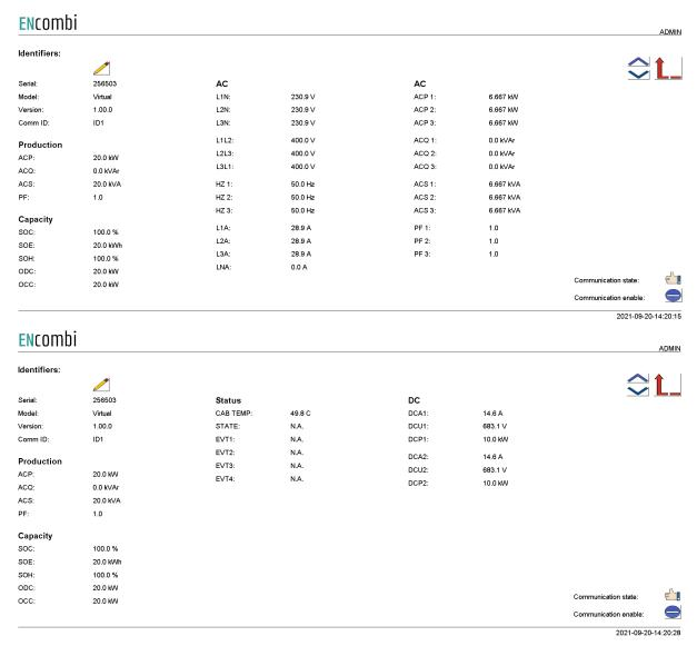
In the upper left corner the label of the inverter can be changed. In the lower right corner communication status for the specific inverter is shown. In case the inverter is failing to communicate for whatever reason, communication to that specific inverter can be disabled and enabled again at a later stage on the start/stop button. In the upper right corner it is possible to toggle between the pages.
