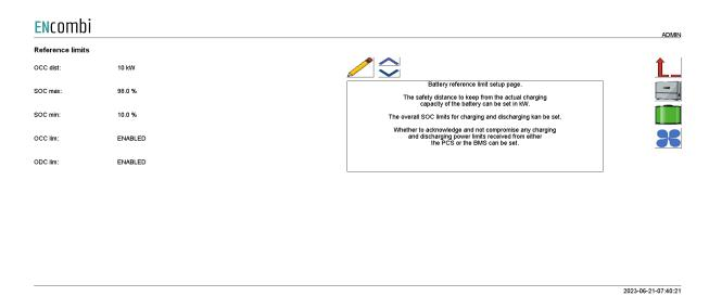
When the battery is charging it is possible to set a safety distance in order to keep the reference close to the actual charginging.
