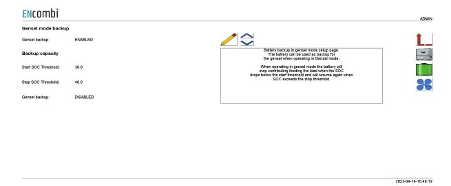
When the battery is operating in genset mode it is possible to let the battery back up if the genset fails. If the genset is failed the battery will continue operating without the genset, if genset backup is enabled.
