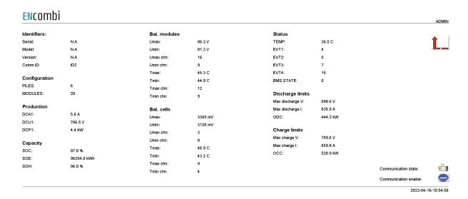
In the lower right corner communication status for the BMS is shown. In case the BMS is failing to communicate for whatever reason, communication to that specific inverter can be disabled and enabled again at a later stage on the start/stop button.
