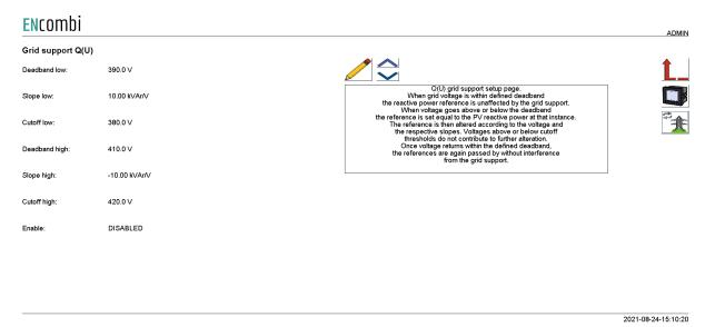
When the grid voltage is within the defined deadband the reactive power reference is unaffected by the grid support. When voltage goes above or below the deadband, the reference is set equal to the PV reactive power at that instance. The reference is then altered according to the voltage and the respective slopes. Voltages above or below cutoff
