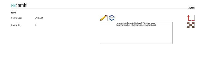
The ECpvX can apply references as Unicast or as Broadcast. The Control ID is used for Unicast.
