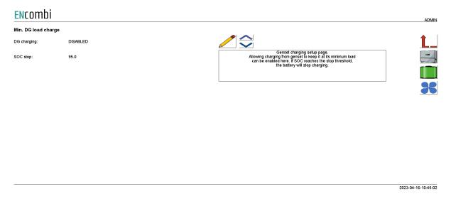
When the battery is parallel with the genset and the load is below the minimum DG load. The battery is able to charge if the SOC is below SOC stop. The battery will start charging and keep the genset at minimum DG load. When the load increases above the minimum DG load the battery will stop charging. If the SOC goes above SOC stop, the battery will stop charging as well.
