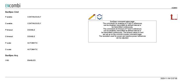
For SunSpec protocol the commands for enabling P and Q references can be disabled, transmitted at a defined interval or be transmitted continuously. The same is the case for the transmission of the fallback timeout values.
