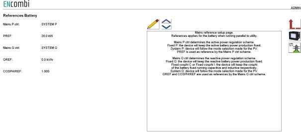
Mains P ctrl determines the active power regulation scheme.
