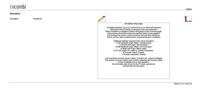
Simulation enables you to try out the ECpvX in an office environment without the need of being connected to any real equipment. When simulation is enabled, a button will appear on the monitoring overview page. Here various stimuli like active and reactive loads can be applied. Run through the various control schemes and see their behavior. Check out how data on plant level to component level is visualized.
