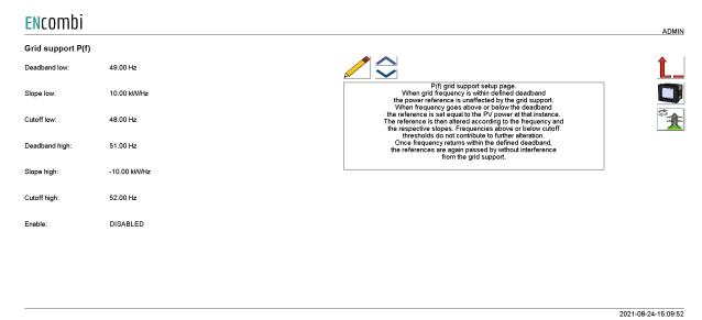
When the grid frequency is within the defined deadband, the power reference is unaffected by the grid support. When frequency goes above or below the deadband, the reference is set equal to the PV power at that instance. The reference is then altered according to the frequency and the respective slopes. Frequencies above or below cutoff thresholds do not contribute to further alteration.
