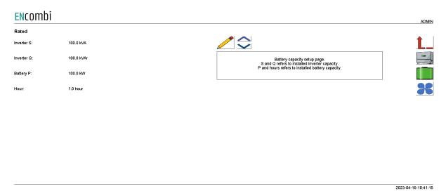
The S and Q ratings refer to the Power Conversion System whereas the P and Hour refer to the installed battery capacity.
