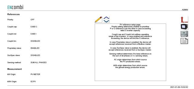
The inverter protocol itself to select in the ECpvX slaves is determined by the make/model of inverters inside their respective inverter clusters.
