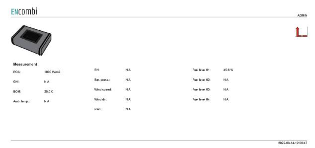
Clicking the up/down navigation buttons will lead to the page below which is displaying the fuel level data.
