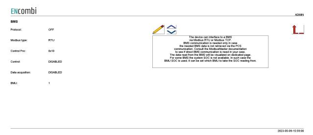
A maximum of 1 BMS is supported by a single ECpvX. The communication can be either Modbus RTU or TCP. Some PCS have communication to the BMS itself and the ECpvX can get the needed BMS information via the PCS thereby making MBS communication obsolete. Check the link below to see which PCS are supported by the ECpvX and which can be handled without the need for separate BMS communication.
