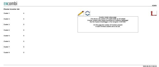
The IP addresses of the superior dataloggers of the inverter cluster must come in a sequential order. Furthermore the Modbus IDs of the inverters in the individual clusters must be sequential and the Modbus ID sequence in each inverter cluster must start at the same value.
