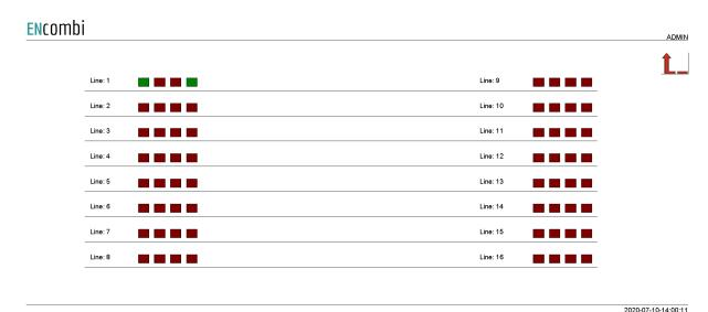
Each builder line consists of four gates. The status of the gates are represented by the color. Red means that the gate is false and green that the gate is true.
