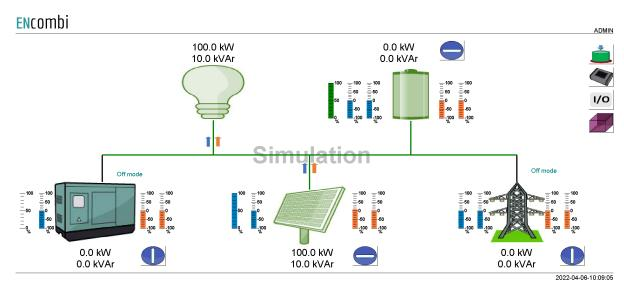
If the genset, PV, battery or utility symbol is grayed out, it means that no configuration for sensing of the associated power is made and therefore the source is interpreted as not being present by the ECpvX. The accumulated powers of the three sources as well as total consumptions are displayed.
