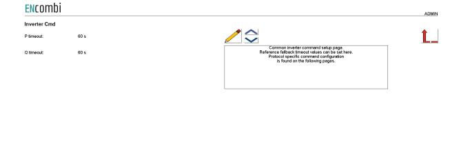
These settings are common for all inverters and may or may not apply to the specific inverter make/model selected. Fallback timeouts for reverting to a predefined production level in case of loss of communication can be set up.
