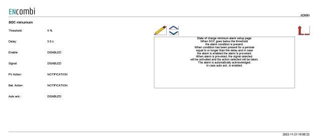
When SOC goes below the threshold, the alarm conditions are present. When the condition has been present for a period equal to or longer than the delay and in case the alarm is enabled, the alarm is provoked. When the alarm is provoked, the signal selected will be activated and the action selected will be taken. The alarm is automatically acknowledged in case auto ack. is enabled.
