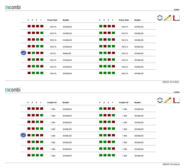
Referring to the ongoing example, as input1 on PV meter1 is active, it means that the RRCR input combination with only input3 being present is true. This is indicated by a check mark. As this line at the same time is enabled, it causes the ECpvX to overrule whatever power reference calculated based on setup made under "Settings" and the current plant status and target the reference dictated by the RRCR instead.
