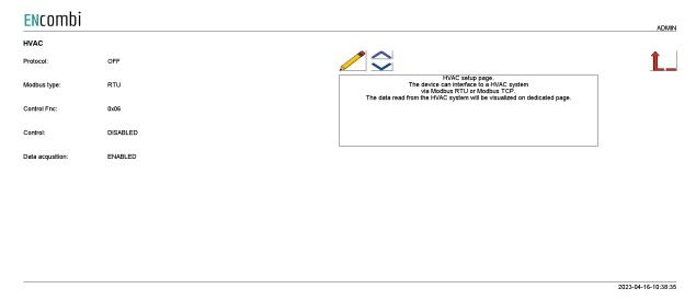
A maximum of 1 HVAC system is supported by a single ECpvX. The communication can be either Modbus RTU or TCP. On the ENcombi website you can see which HVAC systems that are supported. Should your preferred inverter not be on the list already, contact ENcombi to request the adding of it.
