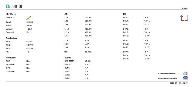
In the upper left corner the label of the inverter can be changed. In the lower right corner communication status for the specific inverter is shown. In case the inverter is
