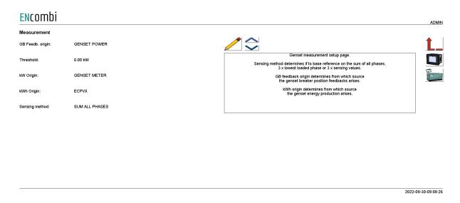
Sensing method determines what power readings to base the calculated references upon. Three options are available.
