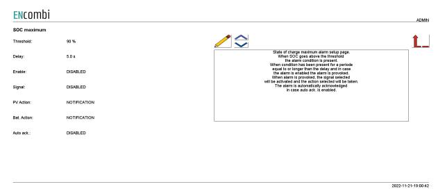
When SOC goes above the threshold, the alarm conditions are present. When the condition has been present for a period equal to or longer than the delay and in case the alarm is enabled, the alarm is provoked. When the alarm is provoked, the signal selected will be activated and the action selected will be taken. The alarm is automatically acknowledged in case auto ack. is enabled.
