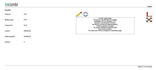
A maximum of 32 inverters is supported by a single ECpvX. In case more than 32 inverters are to be controlled, multiple ECpvX can be stacked to work together. This is discussed in a separate chapter later in this document. All inverters controlled by a single ECpvX must be of the same vendor and possibly model. The communication can be either Modbus RTU or TCP.
