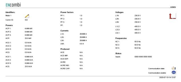
In the upper left corner the label of the meter can be changed. In the lower right corner communication status for the specific PV meter is shown. In case the PV meter is failing
