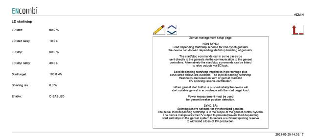
The ECpvX can do load depending start- and stop handling of gensets for two types of genset systems.
