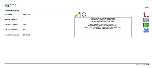
When the battery is operating in grid mode it is possible to let the battery backup if the grid fails. If the grid is failed the battery will continue operating without the grid, if grid backup is enabled.
