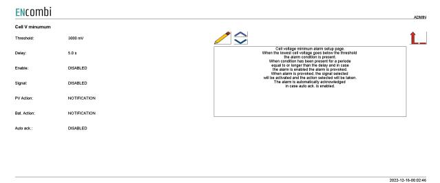
When the lowest cell voltage goes below the threshold, the alarm conditions are present. When the condition has been present for a period equal to or longer than the delay and in case the alarm is enabled, the alarm is provoked. When the alarm is provoked, the signal selected will be activated and the action selected will be taken. The alarm is automatically acknowledged in case auto ack. is enabled.
