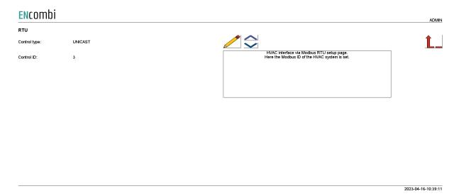
The ECpvX can apply references as Unicast or as Broadcast. The Control ID is used for Unicast.
