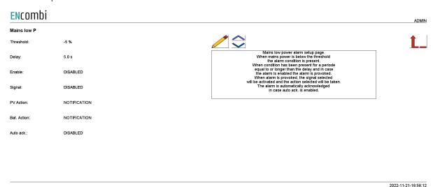
When the mains power is below the threshold the alarm condition is present. When the condition has been present for a period equal to or longer than the delay and in case the alarm is enabled, the alarm is provoked. When the alarm is provoked, the signal selected will be activated and the action selected will be taken. The alarm is automatically acknowledged in case auto ack. is enabled.
