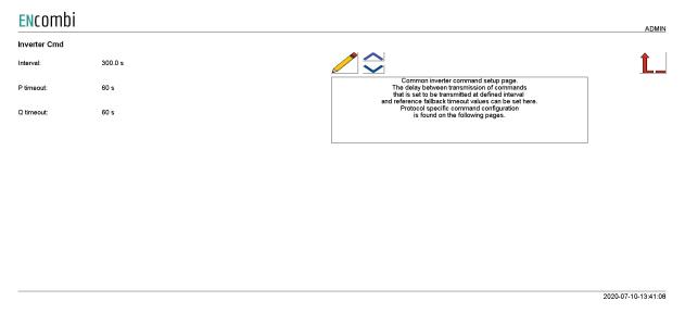
These settings are common for all inverters and may or may not apply to the specific inverter make/model selected. Here the delay between transmission of commands that is set to be transmitted at a defined interval can be set. Furthermore the fallback timeouts for reverting to a predefined production level in case of loss of communication can be set up.
