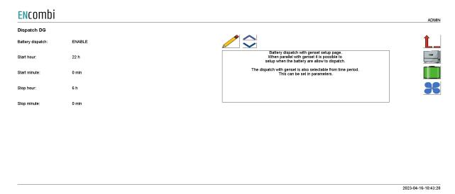
When the battery is parallel with the genset it is possible to select if the battery should be able to dispatch power. It is possible to select if the battery should be able to dispatch all the time or in a specific period of time when parallel to DG. If dispatch is disabled, the battery will still help the genset if the load is bigger than the DG capacity.
