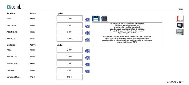
The counters will be incremented automatically by the ECpvX in accordance with operation conditions. The counters are part of the counters backup discussed in the Identifier chapter.
