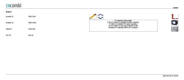
The S and Q refer to the total installed PV inverter capacity whereas the Panel P refers to the total installed PV panel capacity, that is both AC and DC coupled. The PV DC percentage refers to how big a part of the total installed Panel capacity that is DC coupled to the BESS.
