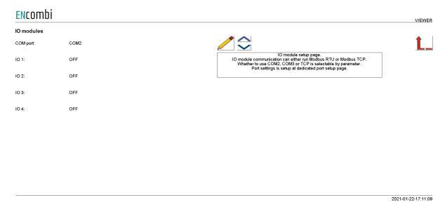
Above page holds the setting up Modbus IO module communication. IO module communication runs either Modbus RTU or Modbus TCP. Whether to use IO modules on COM2, COM3 or TCP is selectable by parameter. A maximum of 4 Modbus IO modules can be connected to the ECpvX. The ECpvX can also read IO data directly from another ECpvX. This is selectable by parameter.
