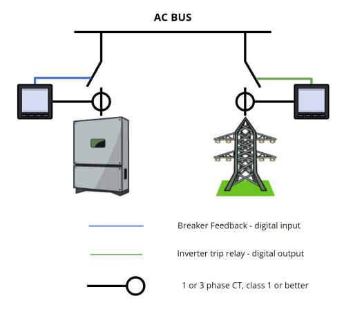
ECpv2 works on single or three phase AC systems.
