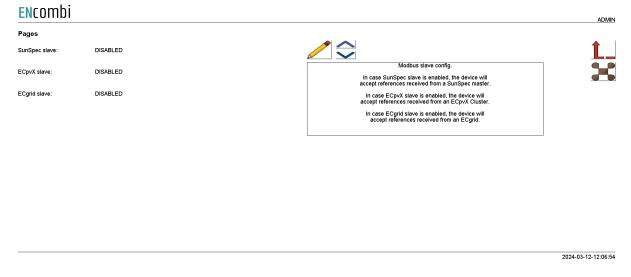
In case SunSpec slave is enabled, the ECpvX will accept references received from a SunSpec master.
