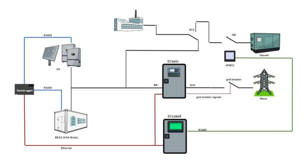
The ECsync Control cabinet's main component is a synchronization relay. The ECsync Control is to be used in conjunction with an external mechanical grid breaker that shall be under the control of the ECsync Control cabinet. The ENcombi EMS ,ECpvX/ECcubeX, will communicate with and control the synchronization relay.
