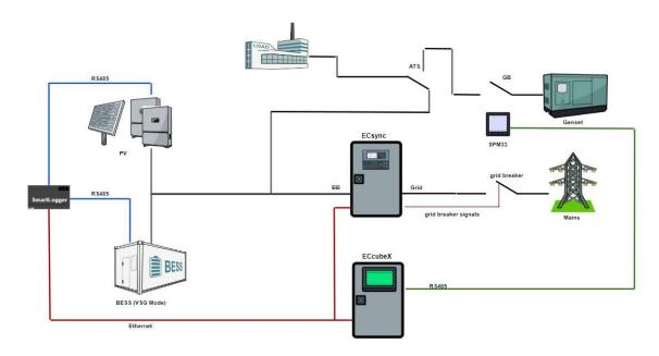
The ECsync Control cabinet's main component is a synchronization relay. The ECsync Control is to be used in conjunction with an external mechanical grid breaker that shall be under the control of the ECsync Control cabinet. The ENcombi EMS ,ECpvX/ECcubeX, will communicate with and control the synchronization relay.
