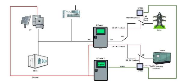
The ECsync cabinet's main components are a mechanical breaker and a synchronization relay. The ENcombi EMS ,ECpvX/ECcubeX, can communicate with and control the synchronization relay.
